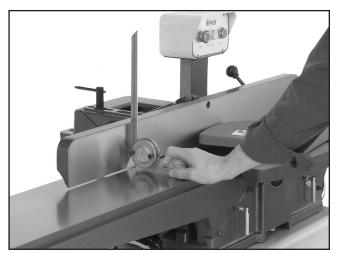
Figure 64. Adjusting fence to 90°.
